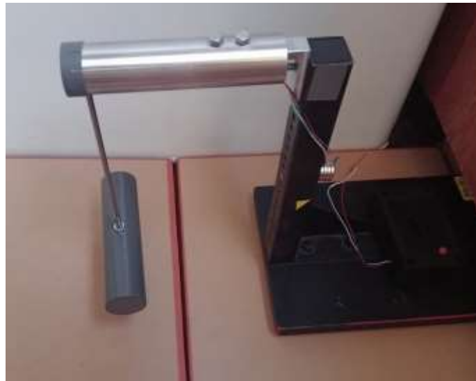
Figure 2: The black scaffolding holds the force cell (hidden in the thick alu tube). At the left side a body (a cylinder in this case) is “hanged” onto the force cell by a thin shaft.
